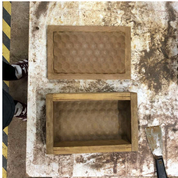
Figure 2.15 // Step 05 - Clean and Construct Mold
